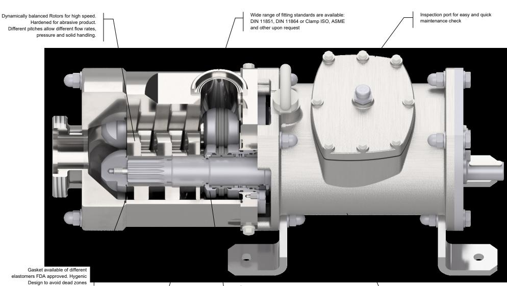
316L Casing material. Screw casing hardening it's optional for very abrasive products. Low clearance to improve the suction capability. Smooth design and wetted part surfaces with Ra<0.8µm Special Hygenic mechanical seal design: single or double acting, depending on the application. Possible to change from single to double with a rebuilt kit, thanks to the modular design of the seals. Special "knife edge" option for abrasive product available
